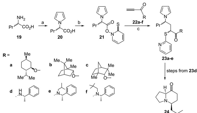
**Scheme 6.** (a) (i)  $\text{SOCl}_2$ , MeOH; (ii) DMTHF, NaOAc, AcOH; (iii) KOH, MeOH; (b) *N*-hydroxy-2-thiopyridone, DCC,  $\text{CH}_2\text{Cl}_2$ ,  $0^\circ\text{C}$  to rt; (c)  $\text{H}_2\text{C}=\text{CHCOR}$ ,  $h\nu$ ,  $\text{CH}_2\text{Cl}_2$ ,  $-40^\circ\text{C}$ .
