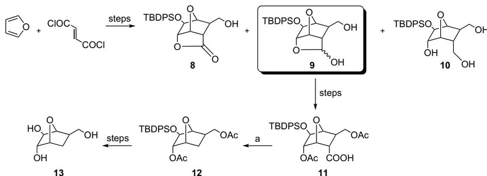
**Scheme 4.** (a) (i) (COCl)<sub>2</sub>, CH<sub>2</sub>Cl<sub>2</sub>, 15 min; (ii) 2-mercaptopyridine *N*-oxide, DMAP, *t*-BuSH, benzene, 1 h, reflux, *hν* (300 W tungsten lamp).
