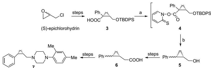
Scheme 3. (a)  $\text{Bu}_3\text{P}$ , 2,2'-dithiobis-(pyridine *N*-oxide), hydrogen donor (THF, benzene or chlorobenzene); (b) (i) radical reaction; (ii) TBAF, THF.
