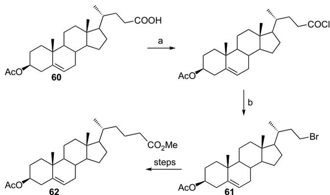
**Scheme 15.** (a)  $\text{SOCl}_2$ ; (b) DMAP,  $\text{CBrCl}_3$ , 2-mercaptopyridine *N*-oxide sodium salt, *h\nu* (73%).
