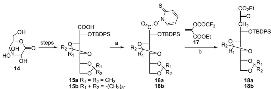
**Scheme 5.** (a) *N*-hydroxy-2-thiopyridone, DCC, CH<sub>2</sub>Cl<sub>2</sub>, 0 °C, 1 h; (b) (i) H<sub>2</sub>C=C(OCOCF<sub>3</sub>)(COOEt), *hν*, –30 °C, 1 h; (ii) satd aq K<sub>2</sub>CO<sub>3</sub>/acetone 1:1, –20 °C to rt, 12 h.
