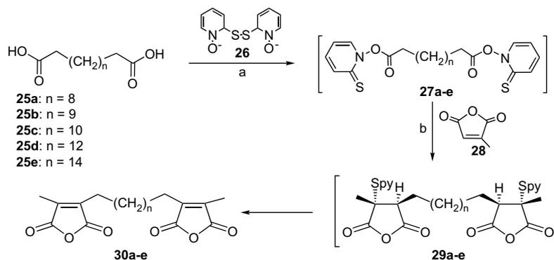
**Scheme 7.** Reagents and conditions: (a)  $\text{Ph}_3\text{P}/2,2'$ -dithiobis-(pyridine *N*-oxide),  $\text{CH}_2\text{Cl}_2$ ; (b) **28**,  $h\nu$ ,  $\text{CH}_2\text{Cl}_2$ ,  $10$ – $15^\circ\text{C}$ , 30 min.
