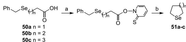
**Scheme 12.** Reagents and conditions: (a) *N*-hydroxy-2-thiopyridone, DCC, CH<sub>2</sub>Cl<sub>2</sub>; (b) *hν*, benzene.
