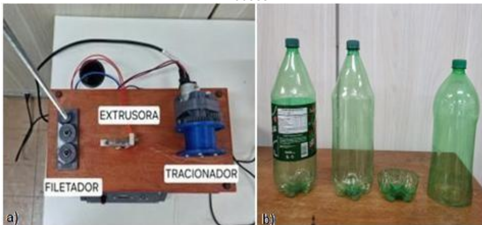
Figure 6. Overview of the Filament Machine and the PET Bottle Cleaning and Treatment Process
