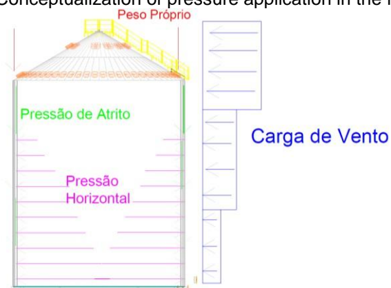
Figure 2. Conceptualization of pressure application in the model silo.
