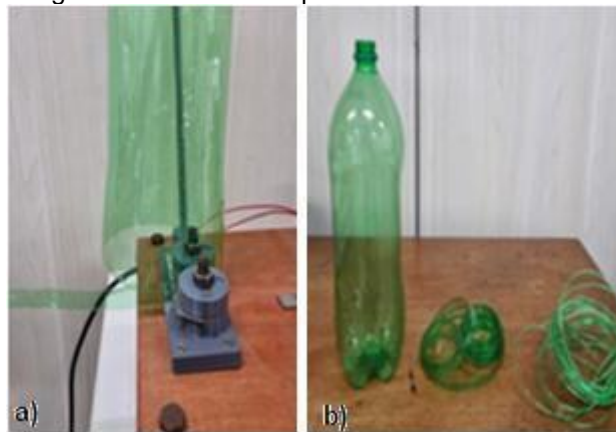
Figure 8. Bottle filation process and PET filament
