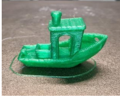
Figure 15. Print of the Benchy model using PET filament
